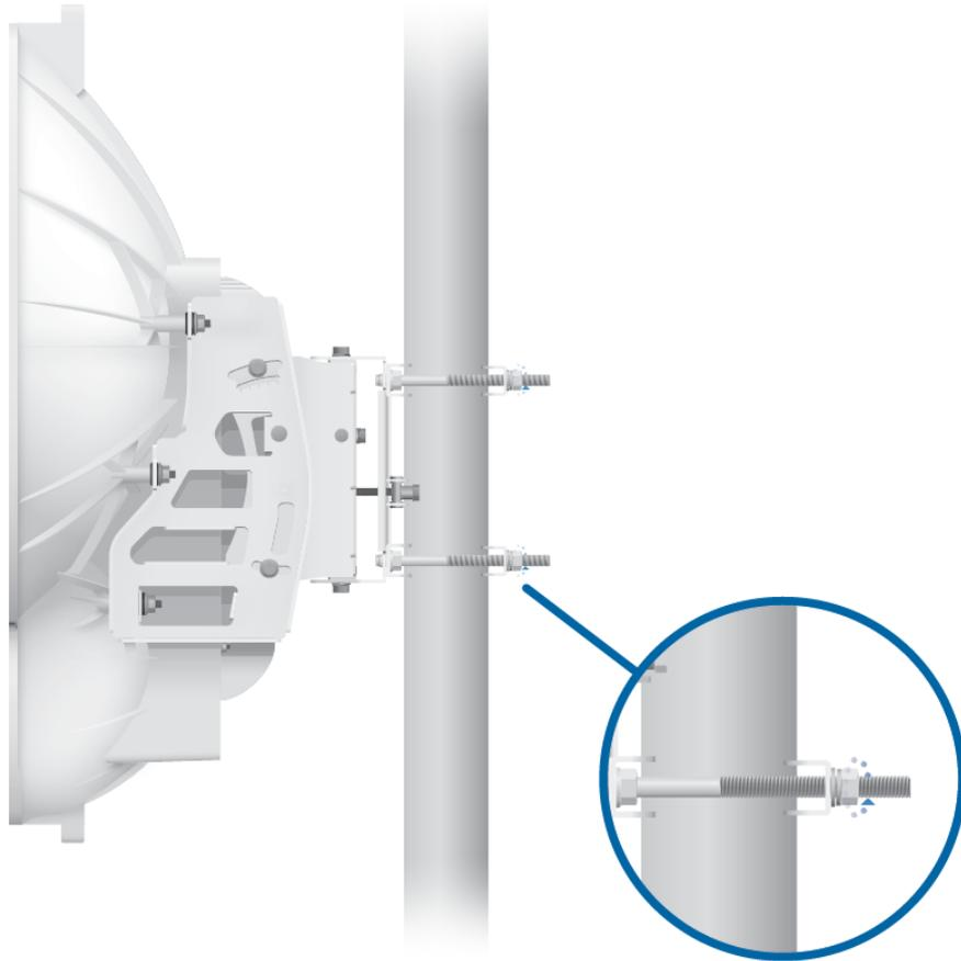
b. Adjust the Pole Mount Bracket and Pole Clamps.
