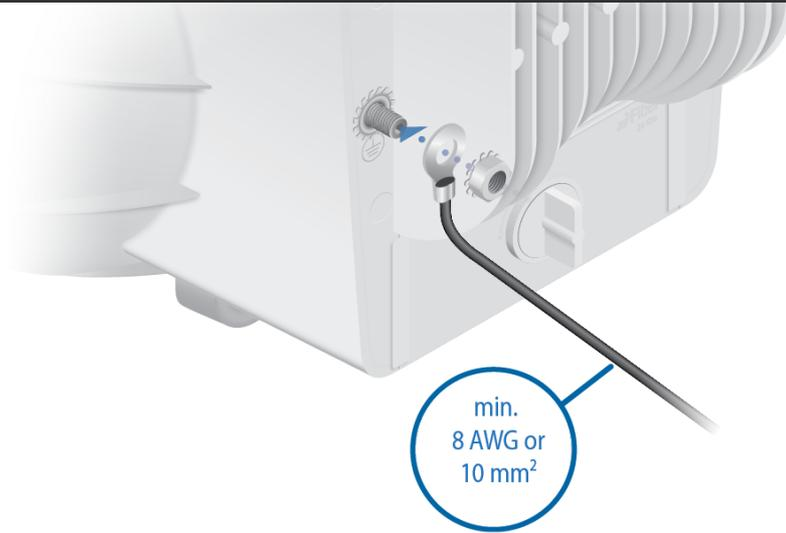
8. Secure the other end of the ground wire to a grounded mast, pole, tower, or grounding bar.
