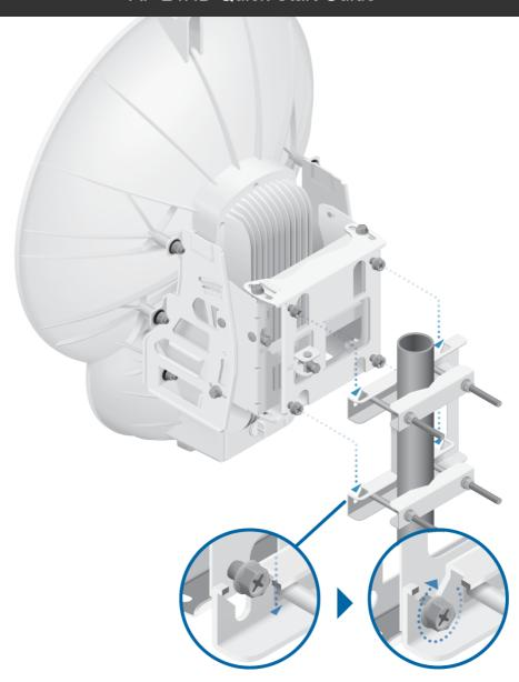
WARNING: To prevent injury, ensure that all four screws are seated and fully tightened.
