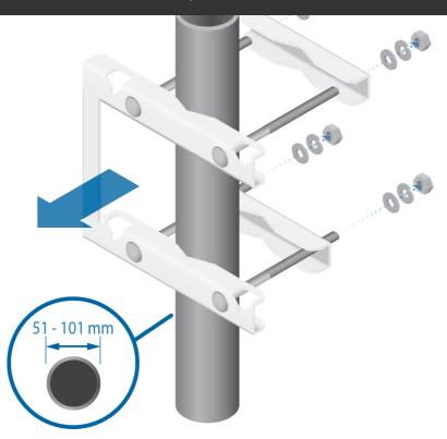
Note: Orient the Pole Mount Bracket around the pole so it is aimed in the direction of the other airFiber AF-24HD.
