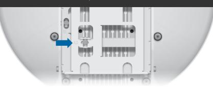
b. Sweep the Elevation (EL) Adjustment Bolt of the Master through its adjustment range.
